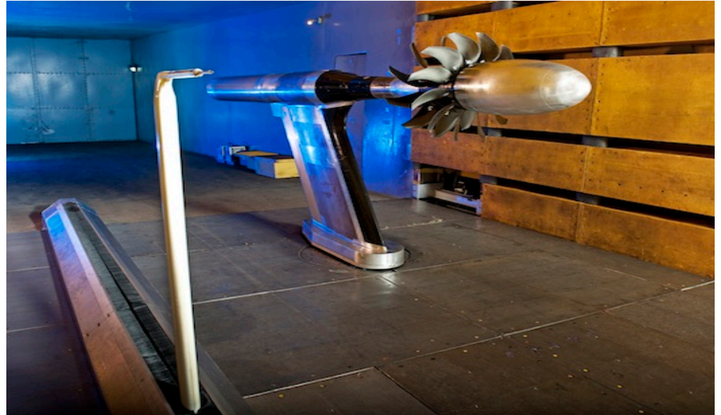
Open Rotor Propulsion Rig installed in GRC's 8x6 and 9x15 Wind Tunnels
